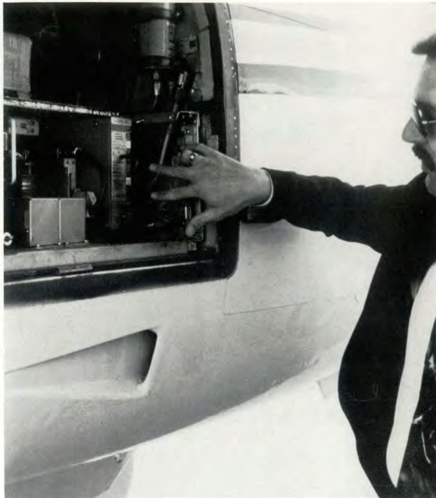
Sunstrand pilot, Mark Johnson, points to the MK VII computer. Weighing 6 pounds, it is the brain of the ground collision warning system.
